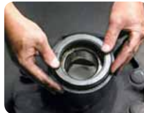
Press the seal into the bore evenly by hand.
