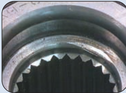
Close-up showing damage to the spindle and incomplete fitting of the inner ring to the spindle.
