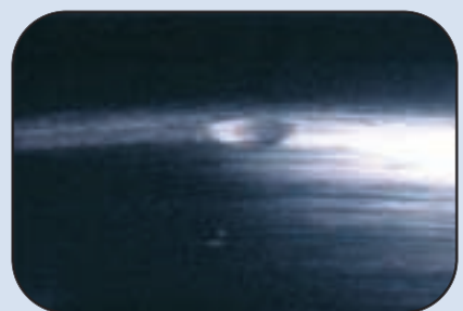
Magnification of a raceway: imprint due to the over-rolling of a damaged ball
