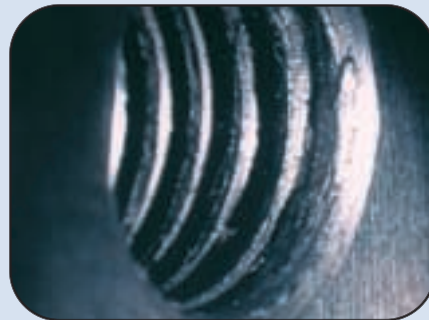
View of a damaged threaded hole
