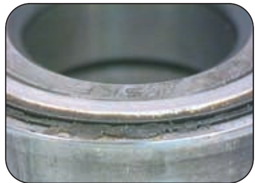
Detail of picture at left showing grease leakage.
