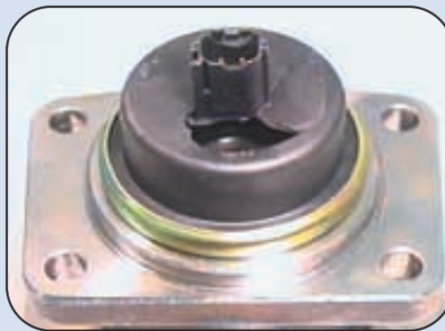
ABS cup is broken due to incorrect handling or improper fitting.
