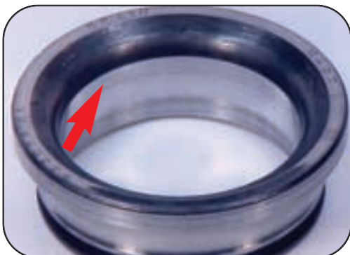
Sign of rotation on the inner ring bore diameter (shiny surface).
