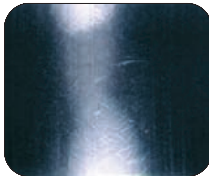
Magnification of a raceway showing imprints due to damaged balls.
