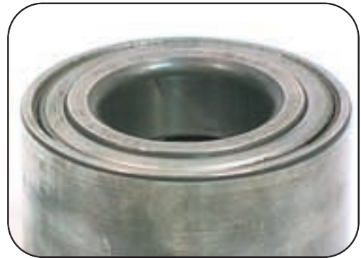
Seal in an oblique position due to wrong fitting during mounting into the knuckle.
