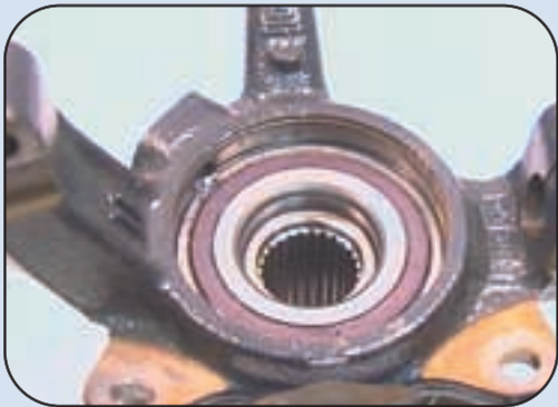
The wrong position of the seal flinger is due to improper fitting on the knuckle and spindle. Always verify lineup of the inner and outer rings.
