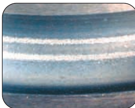
Magnification of a raceway showing signs of damages due to high contact pressure.
