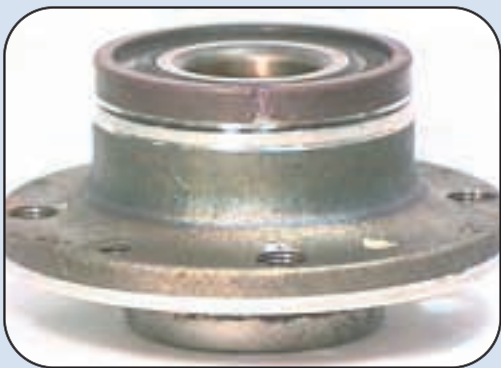
ABS sensor ring broken as a result of an external agent while car is running.
