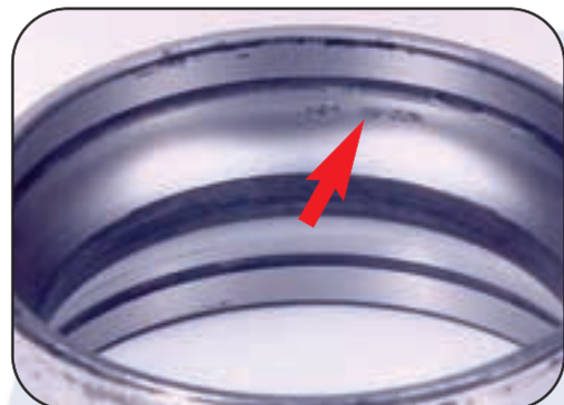
Final flaking on an outer ring.
