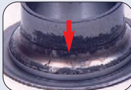
Effects of the water ingress showing oxidation on a raceway.
