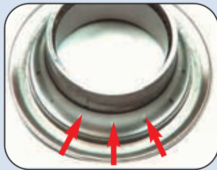
Plastic deformations on a bearing raceway
