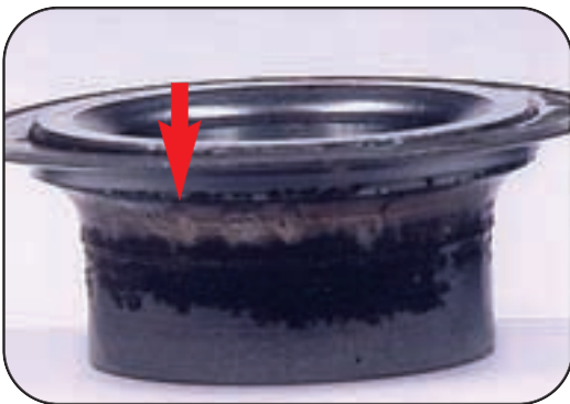
Flinger misalignment on an inner ring.
